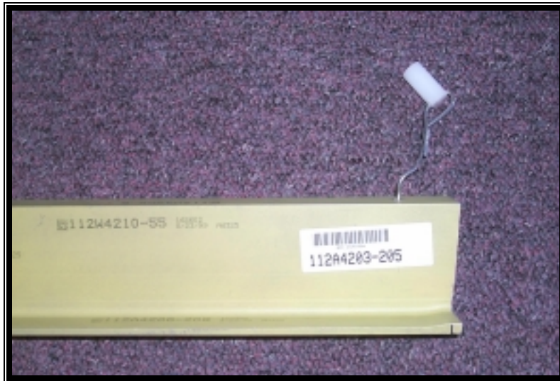
Example part with ink jet part identification, raw stock sticker with 1D barcode and RF tag attached.
