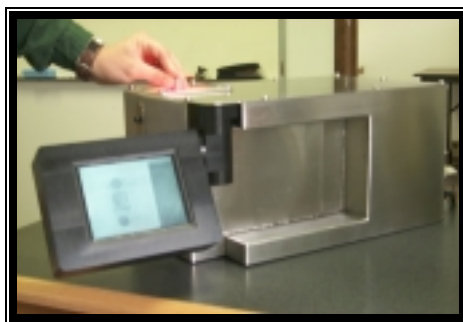
Fixed Station Reader scanning laser-marked tool.
